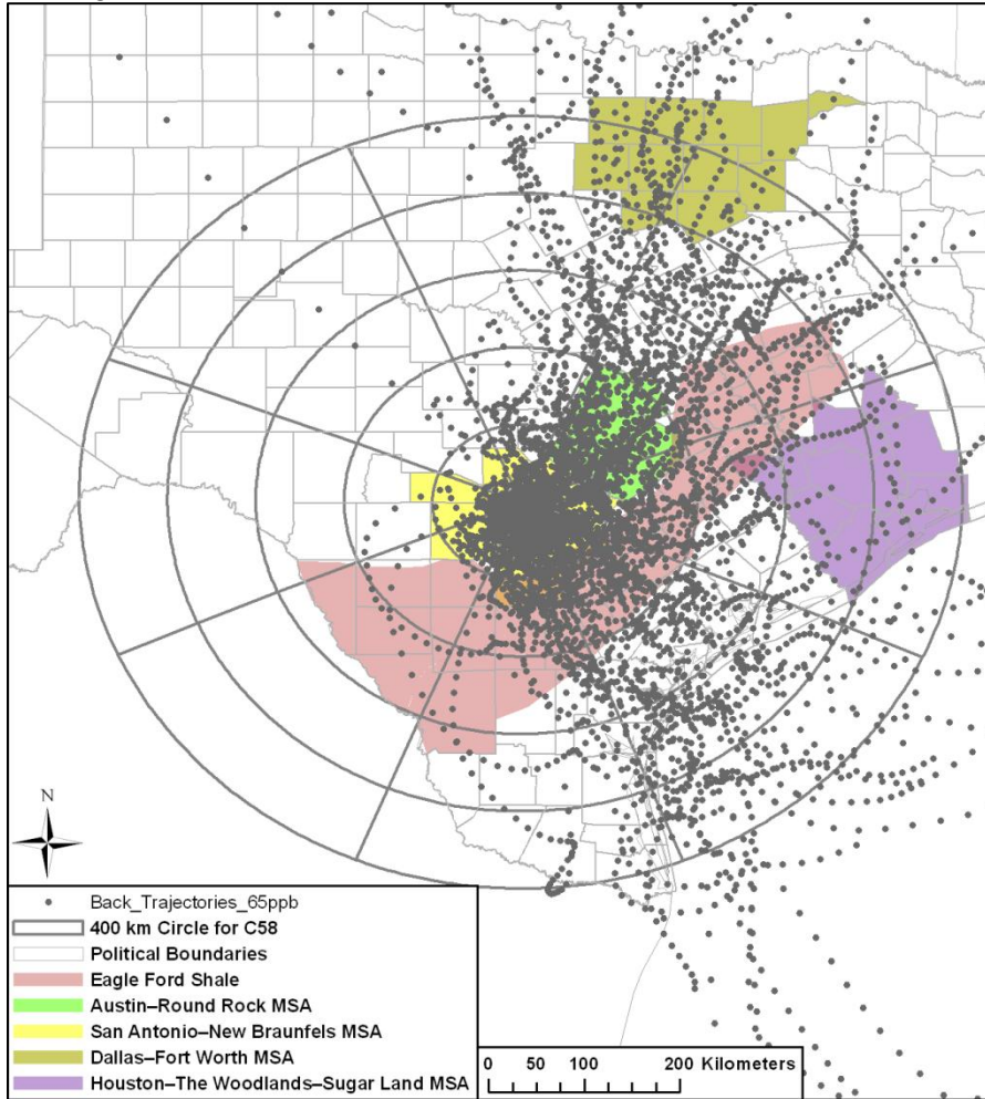
Figure 5-10: Pattern of High Ozone Days > 65 ppb Air Parcel Paths Arriving in San Antonio, 2009 – 2014
